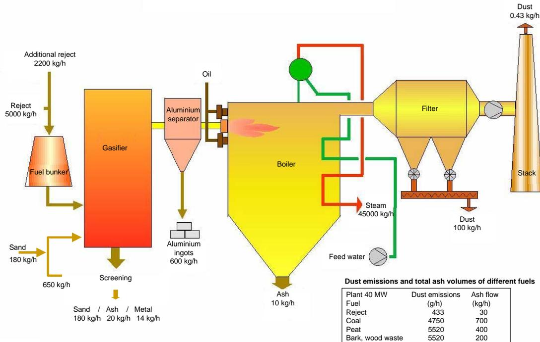
In Corenso's gasification plant, the fibre material in multi-layer packages is recycled in coreboard, the aluminium being recycled as raw material for foil. The remaining plastic is gasified to create energy. The metal and packaging bands in the loads of collected raw material are sent to the metal industry for recycling. Thus, everything is recovered.
