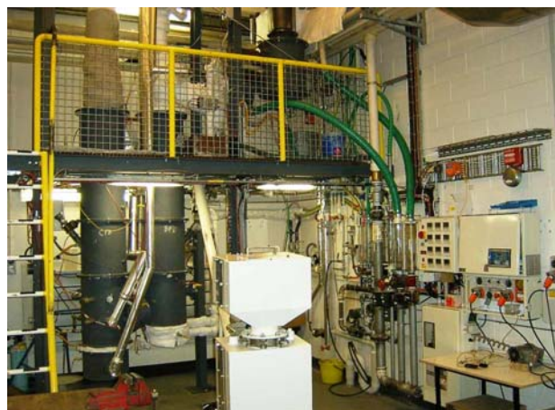
Fig. 7. 100 kW biomass gasifier in CAPE of UoC
